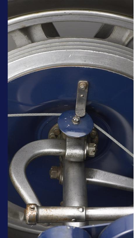
dash. The brake drums were enlarged and the lubrication systems were increased to full pressure feed. With these modifications the Type 37A scored a top speed of 100 miles per hour, making it very successful on the voiturette racing circuit.
